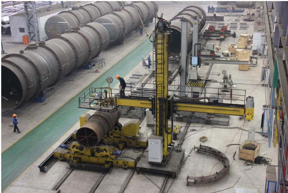
**Welding manipulator used in pressure vessel industry**
