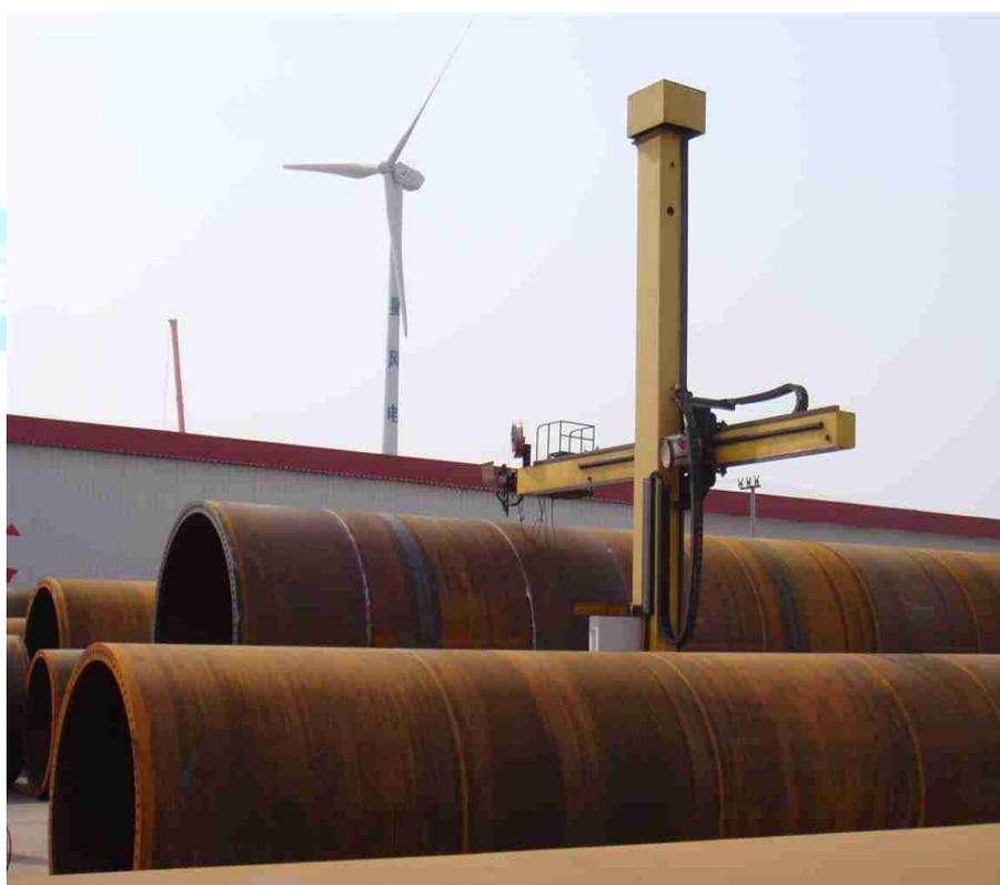
**Welding manipulator used in wind power industry**
