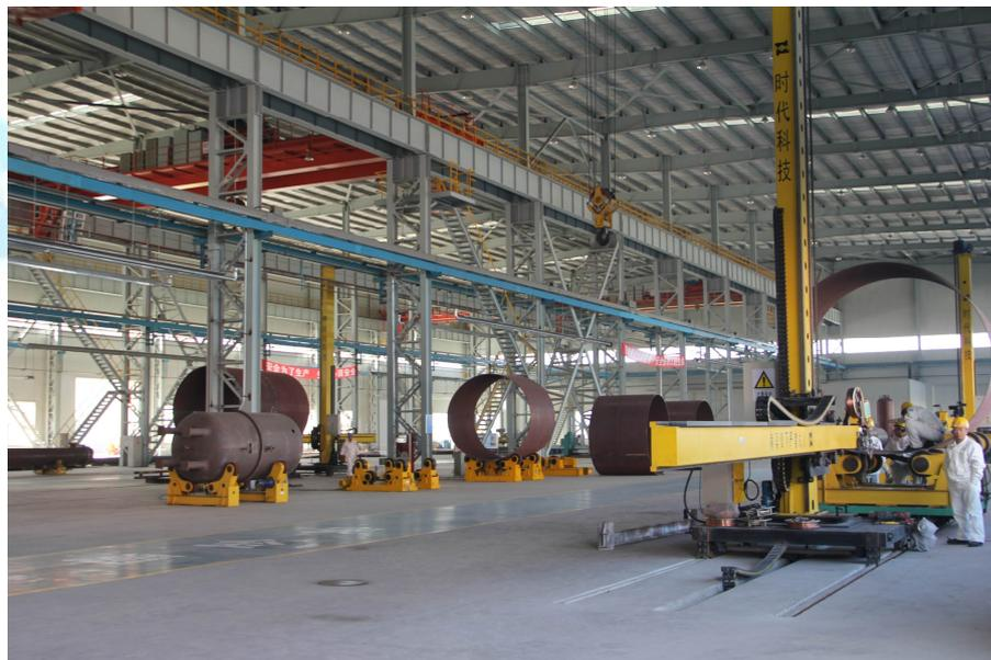
**Welding manipulator used in petroleum industry**
